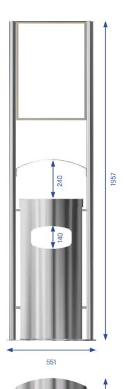
**Description:** Outdoor floor-standing ashtray combined with litter bin, information-frame and cover, self-supporting construction. 6 mm thick base plate, tubular framework. Ashtray and waste combination body with curved fronts and flat sides.
