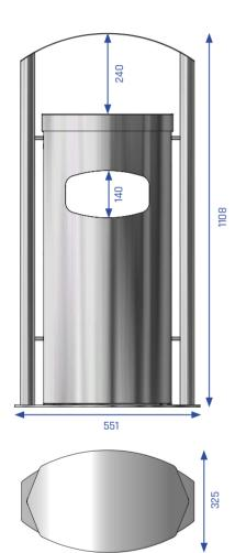
**Description:** Outdoor floor-standing ashtray combined with litter bin and cover, self-supporting construction. 6 mm thick base plate, tubular framework. Ashtray and waste combination body with curved fronts and flat sides.
