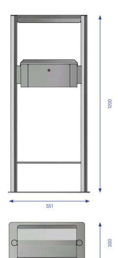
**Description:** Outdoor floor-standing ashtray with cover, self-supporting construction. 6 mm thick base plate (including 4 boreholes for floor mounting), tubular framework with additional round strut (safety feature for visually impaired and blind persons). Ashtray with flat fronts and sides, slitted grid and funnel shaped, oblong insert. The disposal of cigarette packs is not possible.
