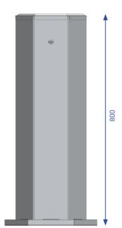
**Description:** Self-supporting construction, base plate (incl. 2 drilled holes), hexagonal column body, removable ash collection tray protected by a 7 mm square lock, with perforated sheet metal web.
