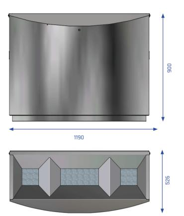
**Description:** Self-supporting, curved fronts, straight back and flat side panels made of stainless steel, secured with an internal construction of galvanized steel, provide great stability. The tops funnel-shaped openings guide waste into the inner liners and are also an elementary part of the fire protection (patented and certified).
