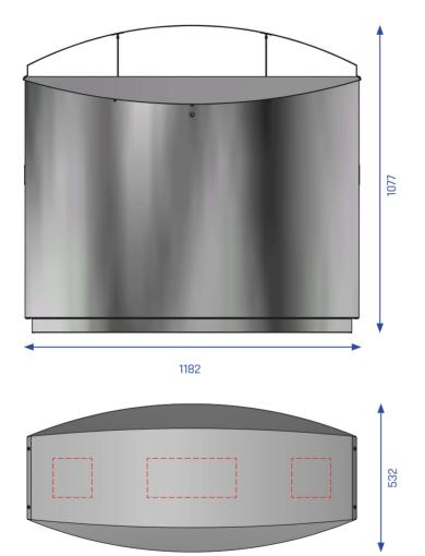
**Description:** Self-supporting, curved fronts and flat side panels made of stainless steel, secured with an internal construction of galvanized steel, provide great stability. The tops funnel-shaped openings guide waste into the inner liners and are also an elementary part of the fire protection (patented and certified).
