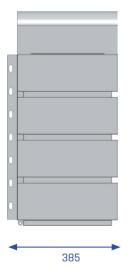
**Description:** Self-supporting body, with four straight sides, in the optics of four rings stacked on top of each other. Flat cover sloping towards the front, firmly connected to the body. The tilted cover results in 2 different insertion heights. Integrated ashtray with stainless still grid (stub-out surface), Separated collection of ashtray contents, detached from waste collection. A U-shaped profile on the back of the body for universal mounting on round as well as square posts.
