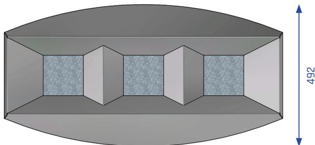
**Description:** Self-supporting, curved fronts with integrated transparent acrylic panels and straight stainless steel side panels, secured with an internal construction made of galvanized steel, provide stability. The funnel-shaped openings of the top guide waste into the inner liners.
