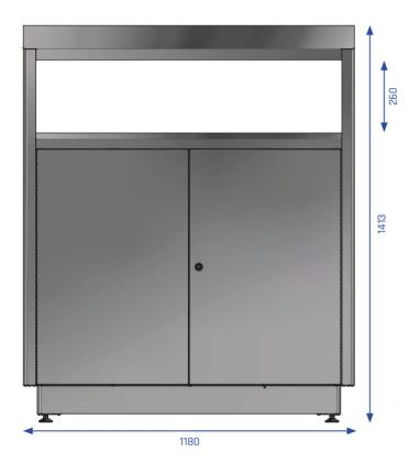
**Description:** Self-supporting, straight exterior walls incl. rounded corner profiles and a cover construction made of stainless steel, fastened with a galvanized interior construction, provide great stability. The funnel-shaped openings on the top of the container guide the waste into either a bag holder (version 1) or a galvanized inner liner, which also serves as a bag holder (version 2).
