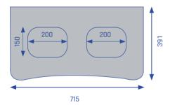
**Description:** Wall-type version made of nickelfree stainless steel, with inwardly curved front, flat top and straight back (made of galvanised steel). Recommended for indoor use.
