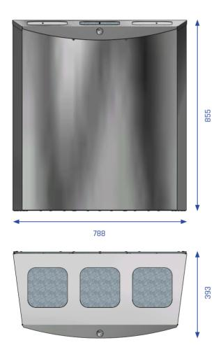
**Description:** Self-supporting, curved fronts and flat side panels made of stainless steel, secured with an internal construction of galvanized steel, provide great stability. The tops openings guide waste into the waste bags which are attached to the included bag holders.
