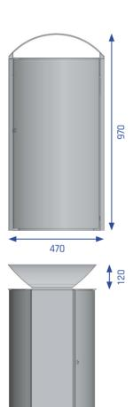
**Description:** Self-supporting, curved, powder-coated galvanized steel outer walls, connected to stable flat side panels. Reinforced door with welded hinges. Two door retention profiles prevent overstretching of the hinges. Doubled cover construction with welded insertion-plates that guide waste into the waste bag. The inner liner or drip tray is sealed.
