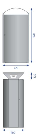
**Description:** Self-supporting, curved, powder-coated galvanized steel outer walls, connected to stable flat side panels. Reinforced door with welded hinges. Two door retention profiles prevent overstretching of the hinges. Doubled cover construction with welded insertion-plates that guide waste into the waste bag. The inner liner or drip tray is sealed.
