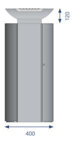
**Description:** Self-supporting, curved, powder-coated galvanized steel outer walls, connected to stable flat side panels. Reinforced door with welded hinges. Two door retention profiles prevent overstretching of the hinges. Doubled cover construction with welded insertion-plates that guide waste into the waste bag. The inner liner or drip tray is sealed.
