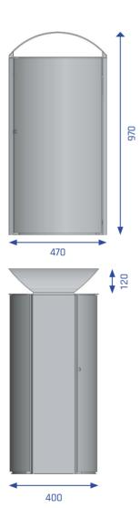
**Description:** Self-supporting, curved, powder-coated galvanized steel outer walls, connected to stable flat side panels. Reinforced door with welded hinges. Two door retention profiles prevent overstretching of the hinges. Doubled cover construction with welded insertion-plates that guide waste into the galvanized inner liner. The inner liner or drip tray is sealed.
