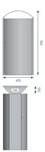
**Description:** Self-supporting, curved, powder-coated galvanized steel outer walls, connected to stable flat side panels. Reinforced door with welded hinges. Two door retention profiles preÂvent overstretching of the hinges. Doubled cover construction with welded insertion-plates that guide waste into the galvanized inner liner. The inner liner is sealed and leakproof.
