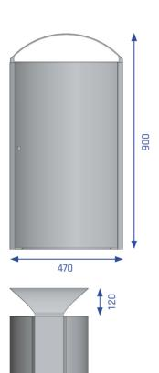
**Description:** Self-supporting, curved, powder-coated galvanized steel outer walls, connected to stable flat side panels. Reinforced door with welded hinges. Two door retention profiles prevent overstretching of the hinges. Doubled cover construction with welded insertion-plates that guide waste into the galvanized inner liner. The inner liner or drip tray is sealed.
