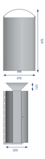
**Description:** Self-supporting, curved, powder-coated galvanized steel outer walls, connected to stable flat side panels. Reinforced door with welded hinges. Two door retention profiles prevent overstretching of the hinges. Doubled cover construction with welded insertion-plates that guide waste into the galvanized inner liner. The inner liner or drip tray is sealed. A U-shaped profile on the back and underneath, for universal attachment to round and square posts, increases stability.
