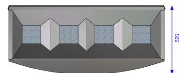
**Description:** Self-supporting, curved fronts, straight back and flat side panels made of stainless steel, secured with an internal construction of galvanized steel, provide great stability. The tops funnel-shaped openings guide waste into the inner liners and are also an elementary part of the fire protection (patented and certified).
