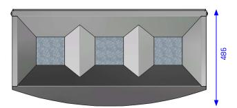
**Description:** Self-supporting, curved fronts, straight back and flat side panels made of stainless steel, secured with an internal construction of galvanized steel, provide great stability. The tops funnel-shaped openings guide waste into the inner liners and are also an elementary part of the fire protection (patented and certified).
