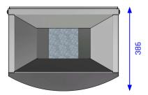
**Description:** Self-supporting, curved fronts, straight back and flat side panels made of stainless steel, secured with an internal construction of galvanized steel, provide great stability. The tops funnel-shaped opening guides waste into the inner liner and is also an elementary part of the fire protection (patented and certified).
