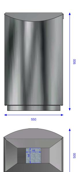
**Description:** Self-supporting, curved fronts and flat side panels made of stainless steel, secured with an internal construction of galvanized steel, provide great stability. The tops funnel-shaped opening guides waste into the inner liner and is also an elementary part of the fire protection (patented and certified).
