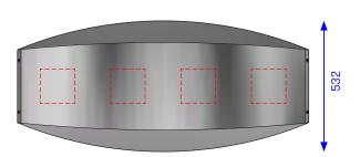
**Description:** Self-supporting, curved fronts and flat side panels made of stainless steel, secured with an internal construction of galvanized steel, provide great stability. The tops funnel-shaped openings guide waste into the inner liners and are also an elementary part of the fire protection (patented and certified).
