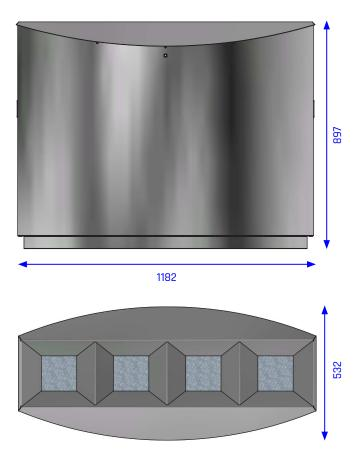
**Description:** Self-supporting, curved fronts and flat side panels made of stainless steel, secured with an internal construction of galvanized steel, provide great stability. The tops funnel-shaped openings guide waste into the inner liners and are also an elementary part of the fire protection (patented and certified).
