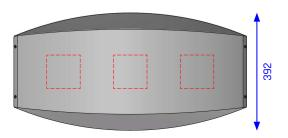
**Description:** Self-supporting, curved fronts and flat side panels made of stainless steel, secured with an internal construction of galvanized steel, provide great stability. The tops funnel-shaped openings guide waste into the inner liners and are also an elementary part of the fire protection (patented and certified).
