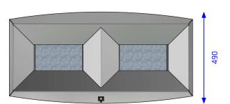
**Description:** Self-supporting, curved fronts and flat side panels made of stainless steel, secured with an internal construction of galvanized steel, provide great stability. The tops funnel-shaped openings guide waste into the inner liners and are also an elementary part of the fire protection (patented and certified).
