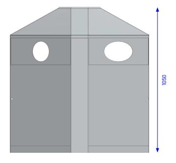
**Description:** Well visible outer walls made of stainless steel. Front openings, suitable for unprotected/ outdoor areas. An integrated, theft-proof ashtray or flat cover on the top is a standard equipment.
